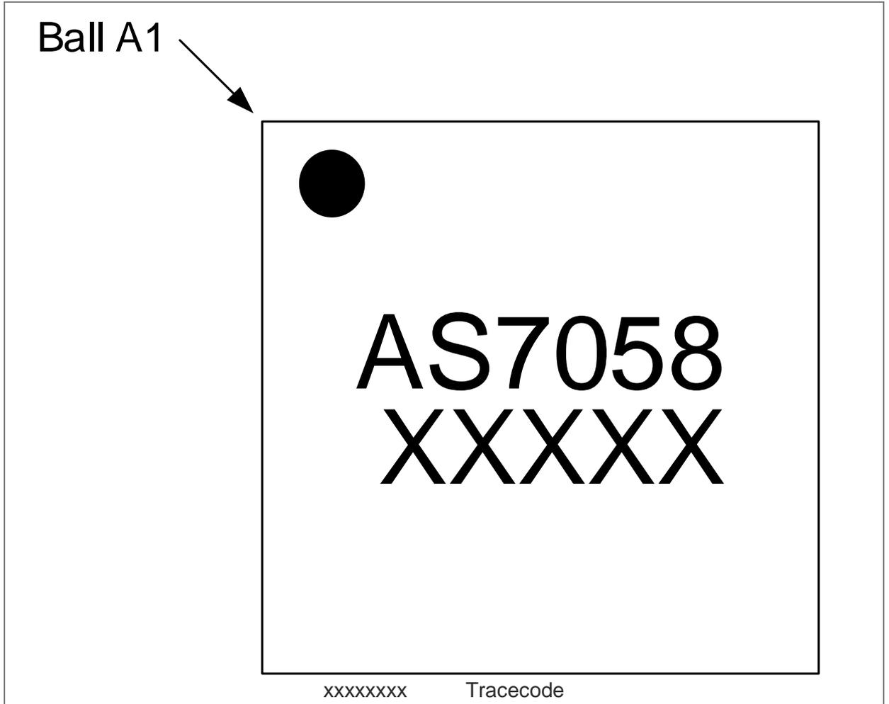
Figure 4: AS7058A WLCSP42 package marking/code
